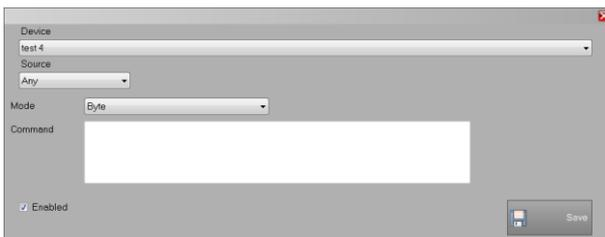
**Mode:** indicate the method of communication with the serial port (ASCII, Byte Hexadecimal,)
