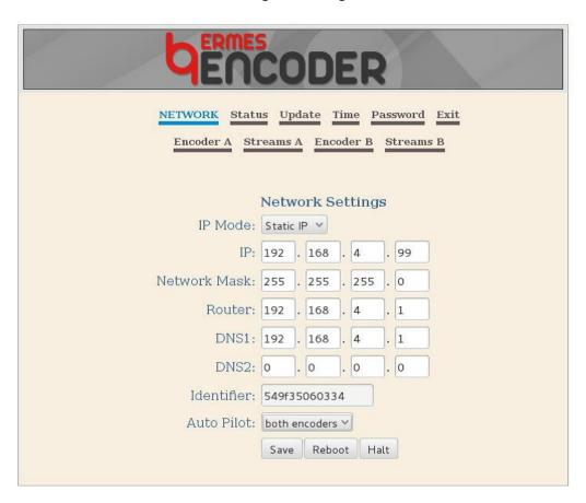
The autopilot option will make the computer work as an encoder automatically when powered up with the settings entered in the Encoder tab, so if power is disrupted, when repowering up the device will start encoding a stream without our intervention. You will have to choose from using only the main encoder (Encoder A) or both encoders at the same time (Encoder A and B).
