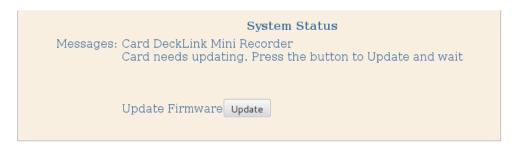
Here we have a very common situation, where the card has been detected or not, and needs a firmware update to work properly. When new BMD drivers are added or brand new cards are plugged in, this is a very common picture. So just connect your computer to the Internet and press Update. In seconds it will start to download the latest Firmware from BMD servers and will burn it on the ROM of the BMD PCIe card to work properly with the latest loaded drivers.
