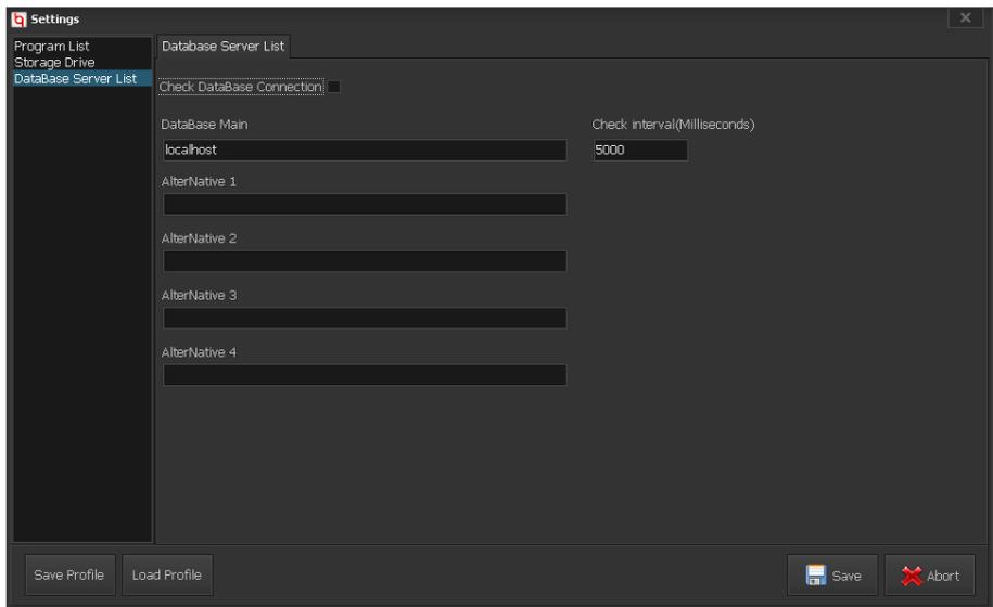
**Check DataBase Connection:** Enables or disables the connection test with the database
